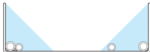
Figure 31 Zones of a cable duct with the highest shielding attenuation
